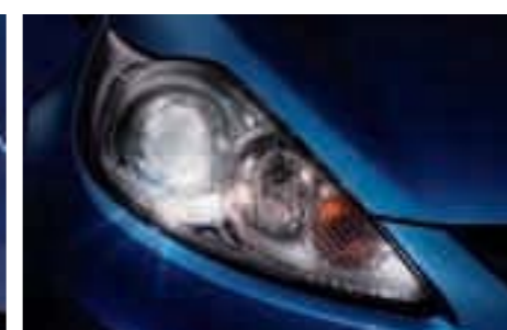
Halogen projector headlights Produce a stronger beam. (Standard)
